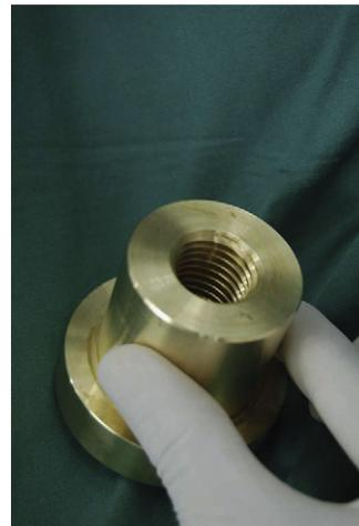
Fig. 2 A view of the device showing the threads for cutting screws.
